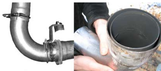
Figure 2.3: The pipe replacing the main silencer, Sil1 .
